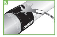
Using a soft propane flame, strip off the separate closure strip. Press the closure strip with the roller over the entire surface, vertically and as firmly as possible onto the shrink sleeve. At the end, the fastening tape must be connected to the entire surface of the shrink sleeve. If necessary, press the edges of the CLRU closure with the roller during the shrinking process.
