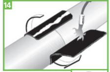
Lay the Superseal product loosely (slack approx. 10% of the joint casing diameter) around the socket and joint casing. Completely remove the release film and briefly heat the hot-melt adhesive at the end of the shrink sleeve
