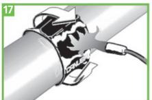
Proceed with the shrinking process with a soft propane gas flame first on the sleeve, then on the jacket pipe until Superseal is smooth and bubble-free and the adhesive has flow out on both sides. The glue must be melted once fingertip test. At the end of the shrinking process, while the glue is still liquid, press down the overlapping area vertially with the roller.
