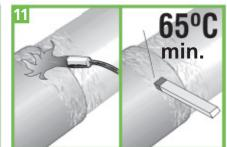
Preheat the entire sealing surface to at least 65°C with a soft propane flame. Check using, for example, a digital thermometer or temperature stick.
