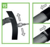
Heat the adhesive side of the closure strip until it is shiny and sticky. Then press the closure onto the overlap with the roller.
