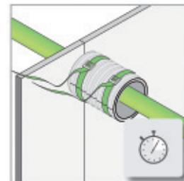
2. Fix the half-shells with a fastening strap or steel wire. Make sure the curing time is not less than three hours before filling in the concrete.
