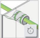
2. Fix the half-shells with a fastening strap or steel wire.
