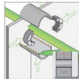
1. Mix epoxy kit and apply epoxy out of the bag on the edge of the half-shells and join the two halves. Smoothen excessive epoxy with a cloth inside and outside. Centre the half-shells with the wall penetration seal if available.
