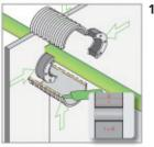
1. Mix epoxy kit and apply epoxy out of the bag on the edge of the half-shells and join the two halfs. Smoothen excessive epoxy with a cloth inside and outside. Centre the half-shells with the wall penetration seal if available.
