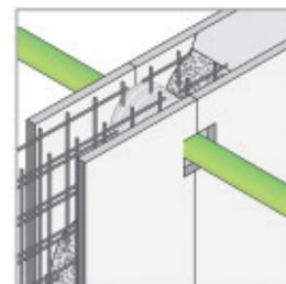
3. Integrate wall sleeve into the casting.
