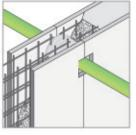
**3.** Integrate wall sleeve into the casting.
