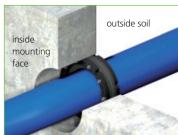
8. Insert the Pressio® seal into the wall and place it flush with the outside of the building.
