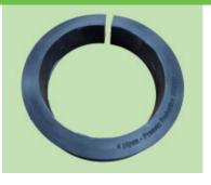
Select the suitable reduction ring for the corresponding diameter of the carrier pipe and insert it into the inner diameter of the seal. For subsequent installation (Type BlackLine), the reduction ring can be split on site using a knife.
