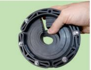
Count the slats to be removed for the corresponding pipe diameter.
