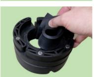
4. To remove the slats, they are pressed through to the back and then cut off with a knife or pulled off by hand.
