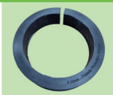
Select the suitable reduction ring for the corresponding diameter of the carrier pipe and insert it into the inner diameter of the seal. For subsequent installation (Type BlackLine), the reduction ring can be split on site using a knife.
