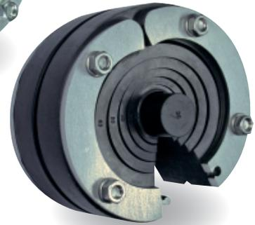
Pressio® Universal Seals can be used as a blind seal or single duct. Because of its soft rubber the Pressio Universal Seals are especially suitable for plastic pipes. The sealing range for the duct of a pipe/cable is stepped with rubber blades and therefore usable for various outside diameters.
