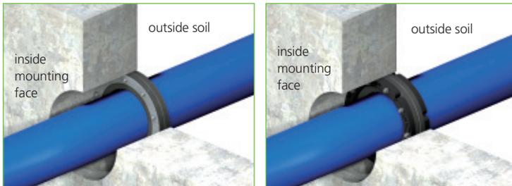
8. Insert the Pressio® seal into the wall and place it flush with the outside of the building.
