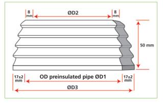
ØD3 **installed** = D1 + 34±4 mm
