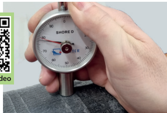
6. Check curing after approx. 60 minutes (approx. Shore D 70°±)
