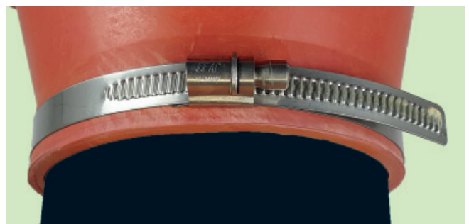
4 pipes stainless steel strap width 20 mm for pipe size OD 75 mm up to 280 mm , Torque value 10 Nm
