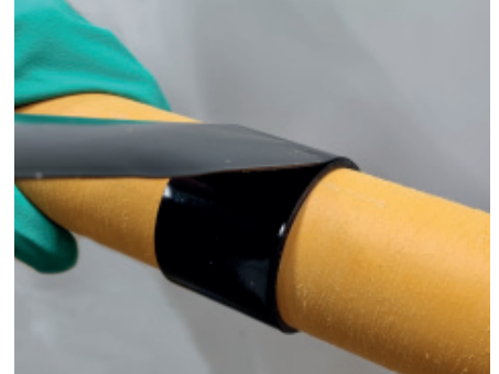
3. Remove sanding residue and wrap anti-sliding tape with 100% overlap in required layers
