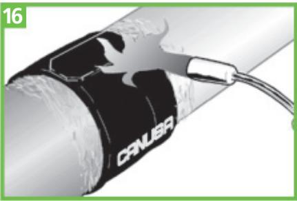
Using a soft propane flame, strip off the separate closure strip. Press the closure strip with the roller over the entire surface, vertically and as firmly as possible onto the shrink sleeve. At the end, the fastening tape must be connected to the entire surface of the shrink sleeve. If necessary, press the edges of the CLRU closure with the roller during the shrinking process.
