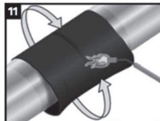
Using the appropriate sized torch, begin at the centre of the sleeve and heat circumferentially around the pipe. Use broad strokes.
