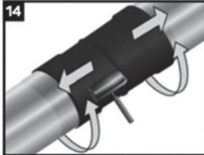
While the sleeve is still hot and soft, use a hand roller to firmly roll the sleeve surface and push any trapped air up and out of the sleeve, as shown above. If necessary, reheat to roll out air.
