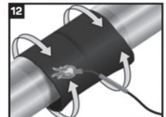
Continue heating from the centre toward one end of the sleeve until recovery is complete. In a similar manner, heat and shrink the remaining side. With a yellow backing, a pink-orange shade will appear when the proper temperature has been reached.
