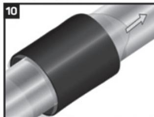
Completely remove the inner release liner from the sleeve and centre the sleeve over the area to be sealed.
