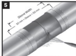
Ensure that the pipe dry before cleaning. Prepare the steel joint area to a minimum of St3 /SP3. Lightly abrade the pipe coating adjacent to the weld area to a distance of 50mm (2") beyond each end of the sleeve width.
