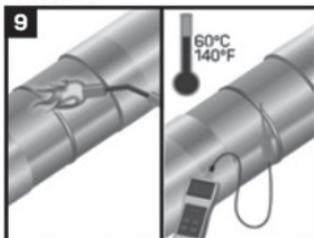
Pre-Heat the joint area to a minimum of 60°C (140°F). Using a temperature measuring device, ensure the correct temperature is reached on the steel and at least 50mm (2") on each side of the sleeve.
