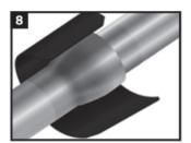
Centre the sleeve over the joint so that the sleeve overlaps between the 10 and 2 o'clock positions. Press the underlap firmly into place and remove the remaining release liner.
