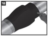
With a gloved hand, press down on the installed sleeve to ensure the backing and sleeve are soft. If there are any cool spots, the sleeve should be reworked with additional heat.
