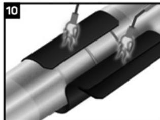
Remove the remaining release liner. Wrap the sleeve loosely around the pipe, ensuring the appropriate overlap. Gently heat the backing of the underlap and the adhesive side of the overlap.
