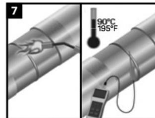
Pre-heat the joint area to  $90^{\circ}\text{C} \pm 5^{\circ}$  ( $195^{\circ}\text{F} \pm 10^{\circ}$ ) with the appropriate propane torch. Using a temperature measuring device, ensure that the correct temperature is reached on the steel and at least 50 mm (2") on each side of the sleeve width. Do not use an intense flame on the mainline coating.
