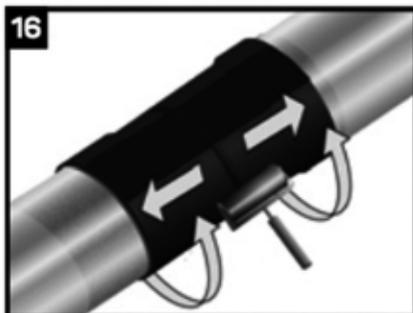
While the sleeve is still hot and soft, use a hand roller to gently roll the sleeve surface and push any trapped air up and out of the sleeve, as shown above. If necessary, reheat to roll out air.
