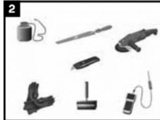
Propane tank, hose, torch & regulator, appropriate tools for surface abrasion, knife, roller, rags & Canusa approved solvent cleanser, digital thermometer with suitable probe, standard safety equipment: gloves, goggles, hard hat, etc.
