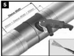
Ensure that the pipe is dry before cleaning. Using a power wire brush, abrade the pipe to a minimum of St3/SP3 (abrasive blast to Sa2.5/SP10 recommended). Lightly abrade the pipe coating adjacent to the cutback area to a distance of 50mm (2") beyond each end of the sleeve width.
