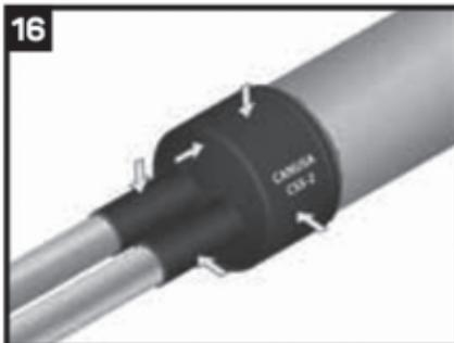
...by heating the entire CSS2 and pressing it firmly with a gloved hand into the profile of the pipe end. Press down with a gloved finger on the shrunk area to ensure the backing and the adhesive are soft. If there are cool spots, the shrink zone should be reworked with additional heat.
