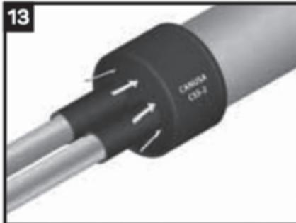
Using a gloved hand, push the CSS2 into the side of the pre-insulated pipe as far as possible.
