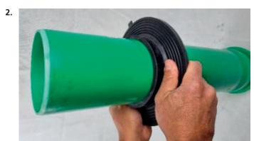
Put wall collar on the medium pipe and center the position of wall sleeve ore core hole.
