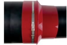
2. Fit the supplied steel strap with max. 10 Nm at the front end of the sleeve on the casing pipe
