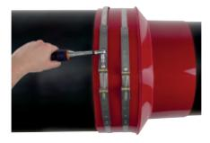
4. Fix second strap with **10 Nm** (smoothen escaping sealant). Repeat step 2 to step 4 on the carrier pipe
