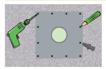
The front of the on-wall sleeve 4 pipes must be installed on a flat, smooth and load-bearing wall surface.
