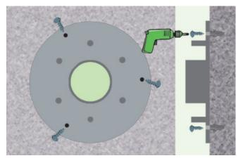
2. Screw the fix on-wall sleeve with the supplied hexagon head screws to the wall.
