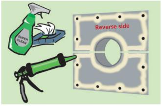
c) (Optional) In case of a split on-wall sleeve version: apply the adhesive on the surface and along the edges of the wall plates. (see image)
