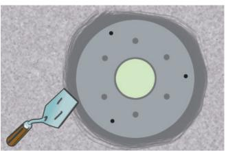
**3.** Use mortar to level the edge from the fixed flange to the wall.
