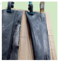
The bonding strips (width approx. 30mm) are thinly coated with the adhesive provided. The adhesive requires approx. 10 - 15 minutes to dry. A finger test is a reliable way to ensure the correct drying time; the adhesive should feel dry but still sticky.
