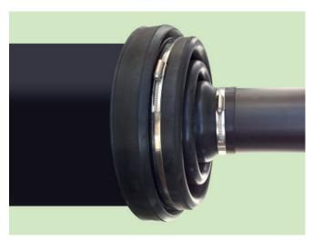
End seals AKT/AWM are made of high quality moulded EPDMrubber. The conic shape of the seal allows a flexible cutting on various pipe diameters. The innovative AWM-seal although the cone is wave-shaped when delivered. AKT/AWM seals are available for a carrier pipes size up to 800 mm. Having only a small number of sizes makes storage easy for our distributors and sales partners..
