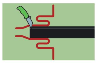
4. If necessary, cut down the seal nozzle to the correct pipe dimension.
