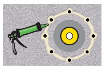
3. Apply **sealing compound** material on the wall with a dispensing gun in a circle around around every screw bore as well as the complete core bore range.
