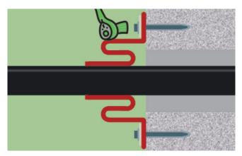
5. Push the side of the Compenseal<sup>®</sup> with flange bore holes first over the carrier pipe, collar facing the wall. After that interlock Compenseal<sup>®</sup> with pressure plate and **spread** emergent **sealing compound**.
