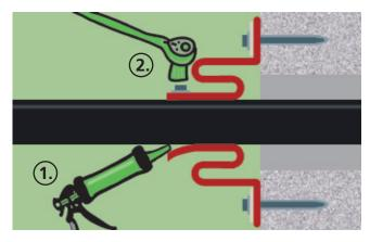
6. Adjust **opening** of the collar to carrier pipe so that a wave shaped expansion zone occurs. **Inject sealing compound** circularly into the collar opening (1) and **fasten bolt strap tightly with 10 Nm** (2).
