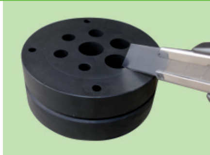
3b. If necessary, cut sealing rubber with a knife.
