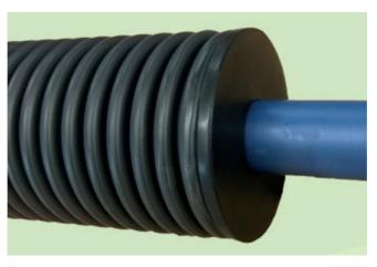
The **Conical Sealing Plug 4 pipes** is designed to seal against low external water pressure. A collar on the wide side makes handling easy and serves as a stop. The extra soft EPDM material  $40 \pm 5$  Shore A makes the application safe and easy. The plug **can be cut to be used as an open product for retrofit applications.**
