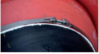
4 pipes stainless steel straps used for pipe sizes up **OD 315 mm** Torque value 10 Nm
