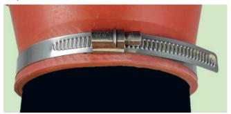
4 pipes stainless steel strap width 20 mm for pipe size **OD 75 mm up to 280 mm,** Torque value 10 Nm
