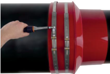
4. Fix second strap with **10 Nm** (smoothen escaping sealant).
